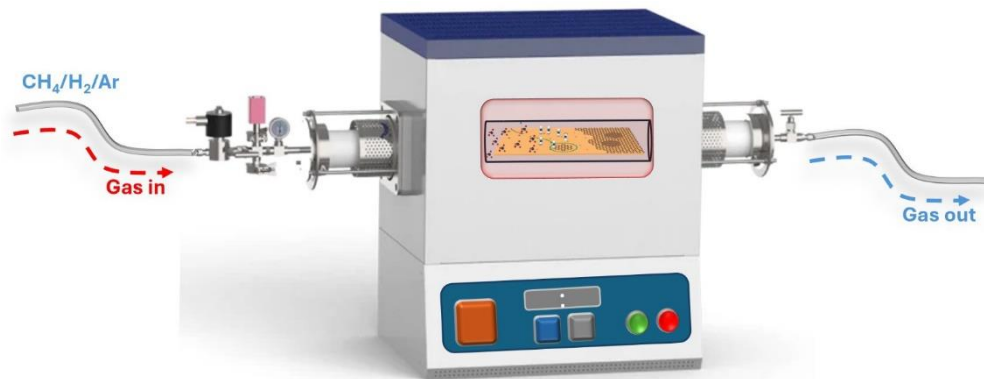
Figure 1. Schematic diagram of the CVD system and growth mechanism of graphene on metallic substrate.
